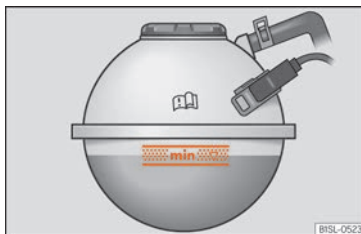
Fig. 161 In the engine compartment: marking on coolant expansion tank.
