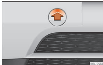
Fig. 42 Right side of the front bumper: remove the cover.
