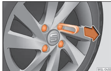
Fig. 31 Wheel: wheel nuts with caps.
