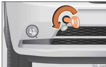
Fig. 43 Right side of the front bumper: towline anchorage in position.
