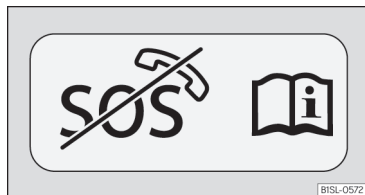
Fig. 133 Sticker subsequently affixed to the vehicle that indicates that the SEAT CONNECT services have been permanently disconnected.
