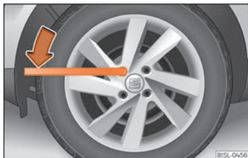
Fig. 33 Wheel change: loosen the wheel nuts.
