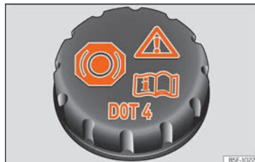
Fig. 63 Engine compartment: brake fluid reservoir cap.
