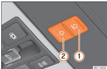
Fig. 129 On the interior roof lining: switches for the sun blind.
