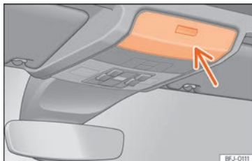
Fig. 174 On the roof console: compartment for glasses.
