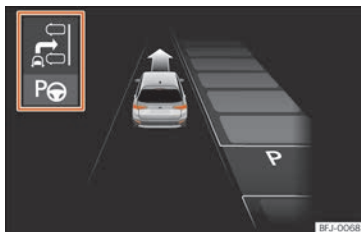
Fig. 282 On the instrument panel display: view of the parking assist system with reduced view.
