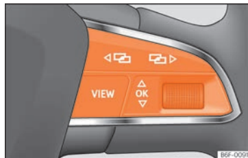
Fig. 64 Right side of the multifunction steering wheel: buttons to the menus and information displays on the instrument panel.
