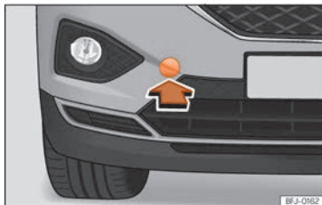
Fig. 48 On the right side of the front bumper: remove the cover.
