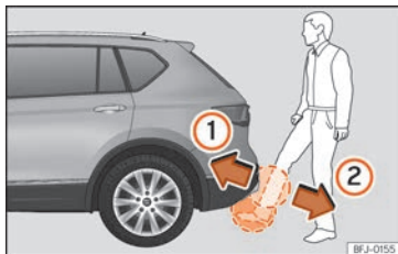
Fig. 87 Rear lid with sensor-controlled opening [Easy Open].
