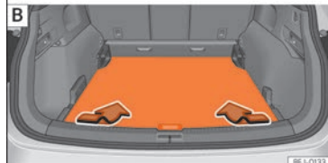
Fig. 129 In the luggage compartment: adjust the height of the variable luggage compartment floor.
