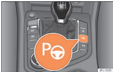
Fig. 281 In the upper part of the centre console: button to switch on the Park Assist system.
