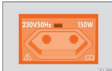
Fig. 151 On the left side of the luggage compartment: 230 volt power socket.
