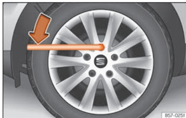
Fig. 38 Wheel change: loosen the wheel nuts.
