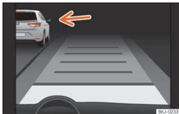
Fig. 267 On the instrument panel display: ACC active, vehicle detected in an outer lane.
