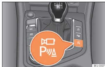
Fig. 296 Centre console: button to manually activate/deactivate the peripheral vision system when combined with the park assist system.
