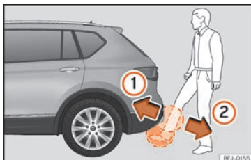
Fig. 83 Rear lid with sensor-controlled opening [Easy Open].
