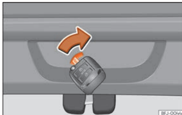
Fig. 84 Detail of the luggage compartment: emergency unlocking
