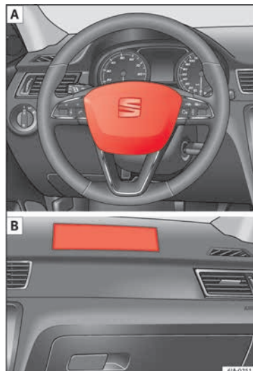
Fig. 15 Driver airbag in the steering wheel and front passenger airbag in the dash panel
