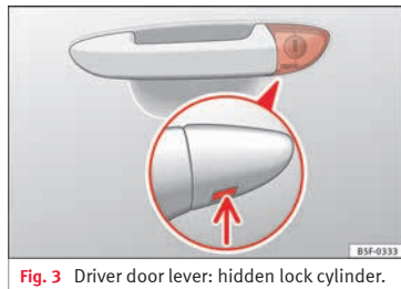
Fig. 3 Driver door lever: hidden lock cylinder.
