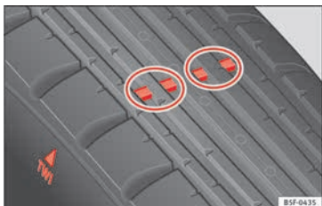
Fig. 213 Side view of tyres with tread wear indicators.
