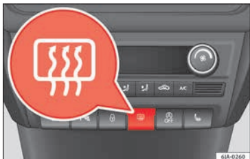
Fig. 137 Heated rear window switch.
