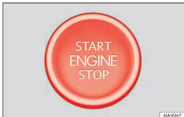
Fig. 173 In the steering column: start-up push button for the Keyless Access lock and start-up system. The layout in right-hand drive vehicles is symmetrical.
