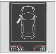
Fig. 41 On the instrument panel display: door open.
