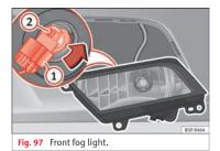
Remove connector » Fig. 97 (1) from the bulb.
