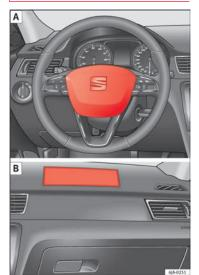
Fig. 15 Driver airbag in the steering wheel and front passenger airbag in the dash panel
