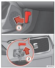
Fig. 7 Unlocking the bonnet.
