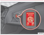
Fig. 17 Front passenger front airbag switch.
