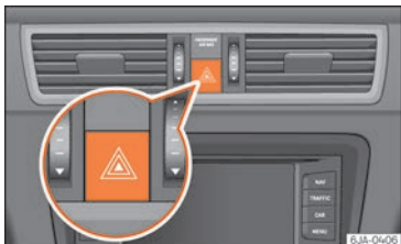
Fig. 32 Dashboard: switch for hazard warning lights.
