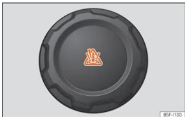
Fig. 52 Engine compartment: coolant expansion tank cap.
