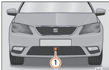
Fig. 224 On the front bumper: radar sensor.
