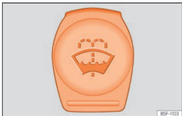
Fig. 54 In the engine compartment: cap of the windscreen washer tank.
