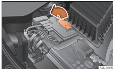
Fig. 248 Battery: opening the cover.
