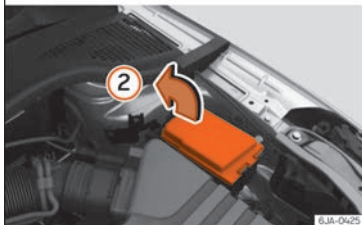
Fig. 88 In the engine compartment: lid of the fuse box - Variant 2
