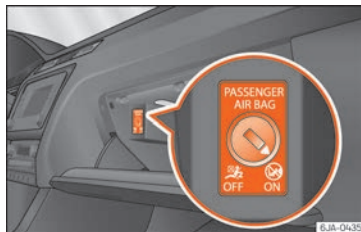
Fig. 20 Front passenger front airbag switch.
