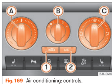
Fig. 169 Air conditioning: controls.
