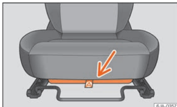
Fig. 149 Driver's seat: storage compartment.
