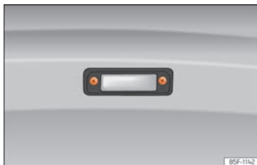
Fig. 108 Removing number plate light
