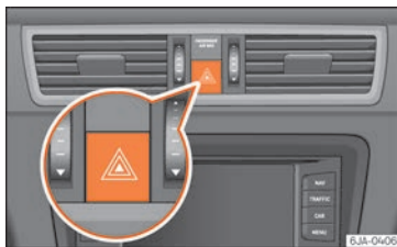
Fig. 133 Instrument panel: switch for hazard warning lights.
