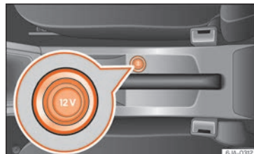
Fig. 154 Centre console: 12 V power socket.
