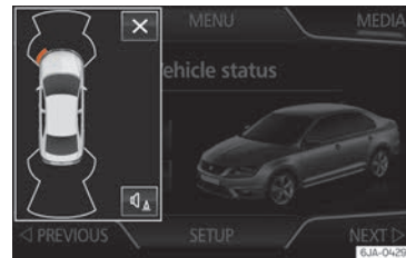
Fig. 228 Miniature indication of automatic activation.
