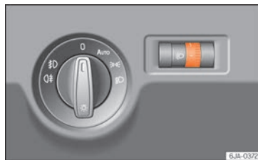
Fig. 130 Instrument panel: light range control.
