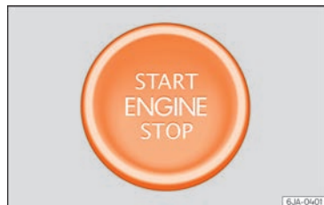
Fig. 212 In the steering column: start-up push button for the Keyless Access lock and start-up system. The layout in right-hand drive vehicles is symmetrical.
