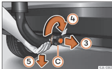
Fig. 240 Unblock the ball-headed bar.
