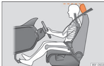
Fig. 73 Correct head restraint position for the driver.
