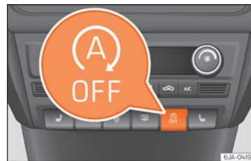
Fig. 221 Instrument panel: Start-stop button.
