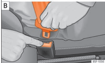
Fig. 14 Positioning and removing the seat belt buckle.
