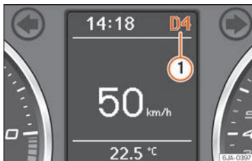
Fig. 217 Information display: selector lever positions.
