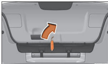
Fig. 8 Luggage compartment: access to manual release.
