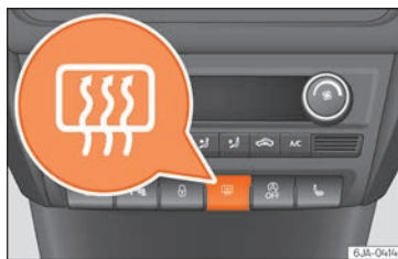
Fig. 137 Heated rear window switch.
