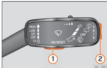
Fig. 38 Windscreen wipers lever: control buttons.
