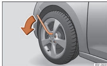
Fig. 63 Tyre change: slacken the wheel bolts. »»
