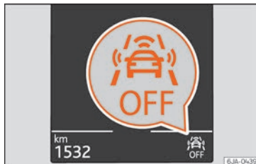
Fig. 225 On the screen of the instrument panel Front Assist switched off message.
