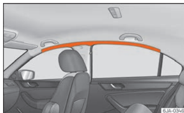
Fig. 23 Location of head-protection airbags.
