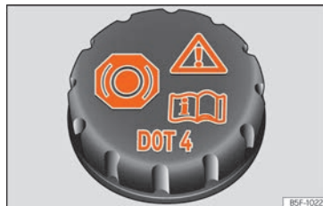
Fig. 53 Engine compartment: brake fluid reservoir cap.
