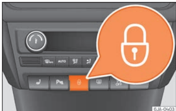
Fig. 4 Centre console: central locking switch.
