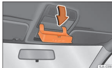
Fig. 156 Close-up of roof panel: storage compartment for glasses.
