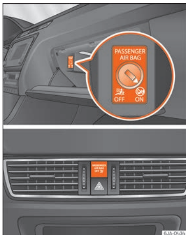
Fig. 82 Front passenger front airbag switch/warning lamp for disabling the front passenger airbag.
